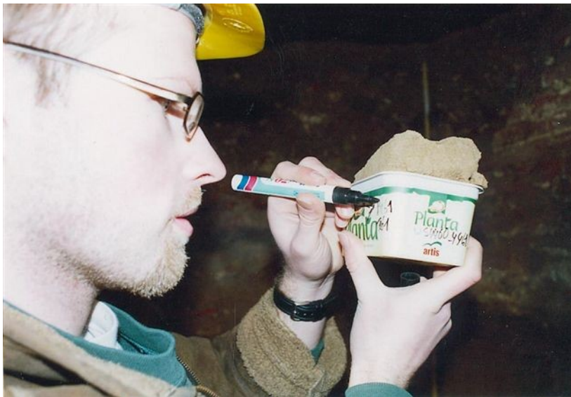
Photo 4: The sample labelling is written on the box, remember to indicate the orientation not only on the box but also on the sample itself by gentle sketching it by arrows (with a knife).
