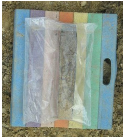
PHOTOS 14-16: Cutting away the surplus soils and packing the box for protection against contamination and chocks, if possible by closing the front and back lids in case of Kubiena like boxes.
