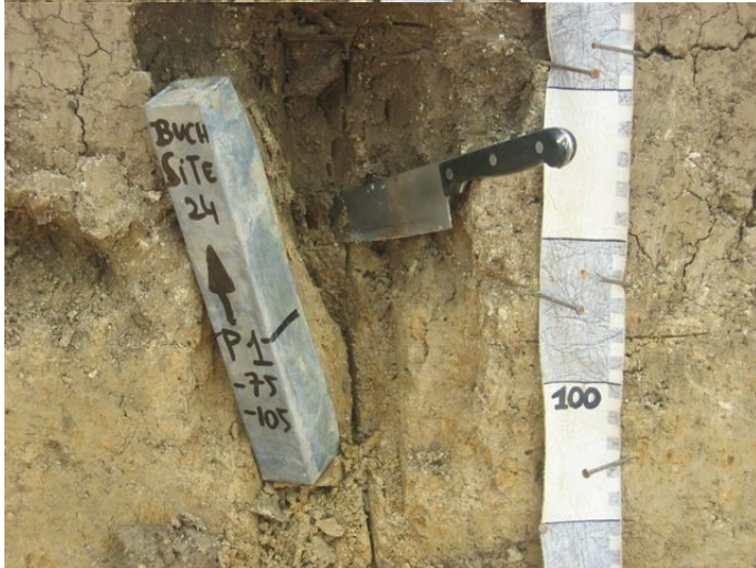
PHOTOS 14-16: Cutting away the surplus soils and packing the box for protection against contamination and chocks, if possible by closing the front and back lids in case of Kubiena like boxes.
