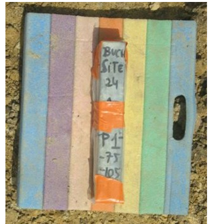
PHOTOS 14-16: Cutting away the surplus soils and packing the box for protection against contamination and chocks, if possible by closing the front and back lids in case of Kubiena like boxes.
