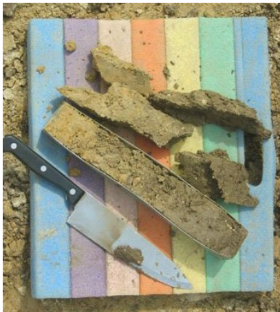
PHOTOS 14-16: Cutting away the surplus soils and packing the box for protection against contamination and chocks, if possible by closing the front and back lids in case of Kubiena like boxes.
